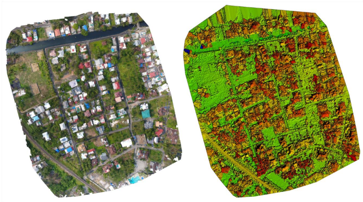
7.7 Aerial 3D flood mapping for Archeology department DSM from pix4dmapper
